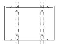
Maximum Load: Uplift load ≤ 2400 Pa Downforce load ≤ 5400 Pa
