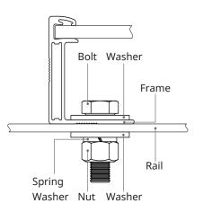
Modules should be bolted at the following hole locations depending on the configuration and loads: Bolting on the short frame side using four standard mounting holes. Mounting rails run perpendicularly to the long frame side. An additional support bar should be placed below the module as shown below.
