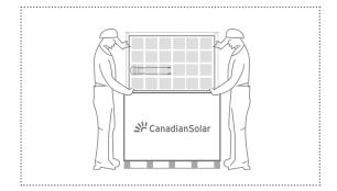
Do not stand, step, walk and / or jump on modules under any circumstances. Localized heavy loads may cause severe micro-cracks at cell level, which in turn may compromise module reliability and void Canadian Solar Inc's warranty.
