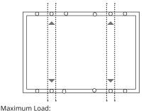
Uplift load ≤ 2400 Pa Downforce load ≤ 5400 Pa
