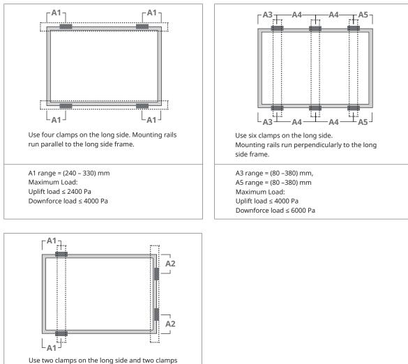
on the short side. Mounting rails run perpendicular to the long side frame.
