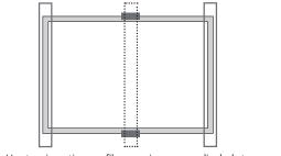
Use two insertion profiles running perpendicularly to the long side frame. An additional support bar should be placed below the module. Use two clamps on the support bar.
