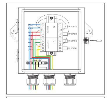
Use the screwdriver to unscrew the nut with position numbers 3 and 5(each contactor) in the contactor, and then insert EPS-R, EPS-S,EPS-T wires and EPS-N wires into the port of contactor(3&5) through the cable nut and tighten them with screwdriver. Use a screwdriver to lock the ground wire on the E-wire copper bar.
