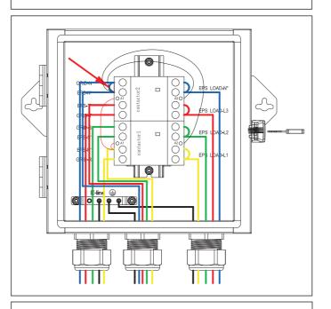
Use the screwdriver to unscrew the nut with position numbers 5 and 7(contactor2) in the contactor, and use 10 AWG wire shorting contacts 2 of 5 and 7 ports and tighten with a screwdriver.
