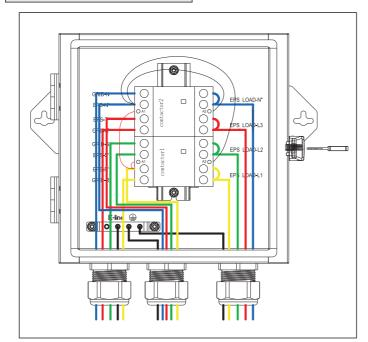
Use the screwdriver to unscrew the nut with position numbers 2, 4, 6 and 8 (each contactor) in the contactor, and the red 10AWG short wire ends were inserted into the contactor port 2 and 4, The Black 10AWG short wire ends were inserted into the contactor port 6 and 8, then insert EPS load-R,EPS load-S,EPS load-T wires and EPS load-N wires into the port of contactor(2&6) through the cable nut and tighten them with screwdriver. Use a screwdriver to lock the ground wire on the Ewire copper bar.
