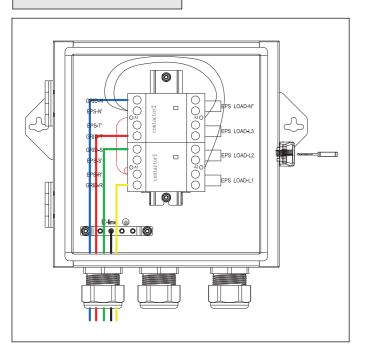
Use the screwdriver to unscrew the nut with position numbers R1 and R7(each contactor) in the contactor, and then insert GRID-R,GRID-S,GRID-T wires and GRID-N wire into the port of contactor(R1&R7) through the cable nut and tighten them with screwdriver. Use a screwdriver to lock the ground wire on the E-wire copper bar.
