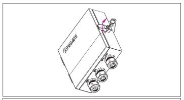
As shown above, please put the key into the Keyhole on the ATS-T right, clockwise rotation of 90°, the lower end of the first lock up gently move Open, remove the lock at the upper end of the buckle, then you can open the cover, Step of locking the cover opposite to the above.
