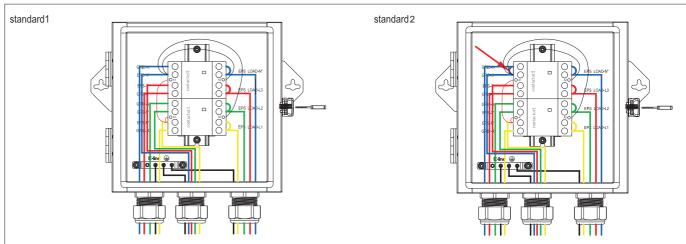
Standard 1 is for general using, and standard 2 is for like Australia where Neutral line can't be switched. When connect with ATS-T, please check which standard is suit for you.
