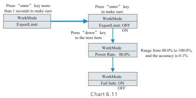
Exportlimit is used for users to control the energy flowing to the grid. If this function is enabled, the feeding power to grid will be equal or less than the setup value. The purpose of the Fail Safe function is to ensure that should any part of the ELS fail, the Active Power exported across the Connection Point will drop to the Agreed Export Capacity or less within the specified time.
