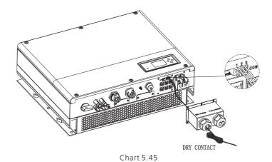
If the cable such as "Dry contact" cable is not used, please do not remove the filler plug from the cable support sleeve.
