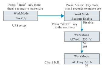
In the back up you can set UPS, including enable or disable (default is enable), AC voltage(default is 230V) and frequency(default site 50HZ).
