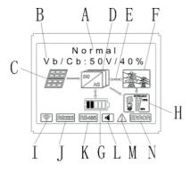
Chart 6.2 Description Location Α State Information В PV input (If you connect two tracks, it will show two. C Otherwise show one) D SPH inverter Ε Power flow line Grid F G Battery (Show the SOC in five grid, Every grid represents 20%) Н Local load Wireless communication J RS 232 Κ RS 485 Buzzer(Reserved) L M Warning Ν Fault
