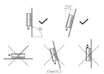
H. Installation position shall not prevent access to the disconnection means. I. In order to ensure machine can run normally and easy to operate, please pay attention to provide adequate space for SPH, please refer to below:
