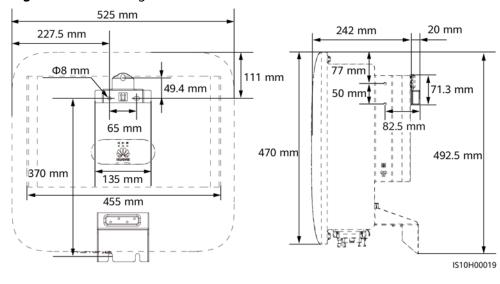
Figure 4-7 Mounting bracket dimensions
