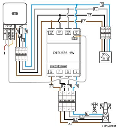
**Figure 5-26** Three-phase, three-wire direct connection (SmartLogger networking)
