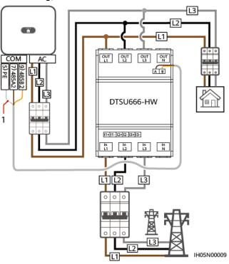
**Figure 5-24** Three-phase, three-wire direct connection (Smart Dongle networking)
