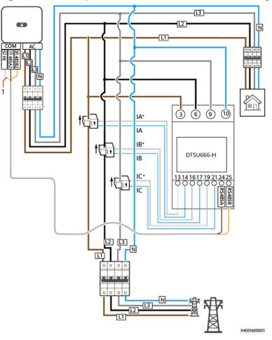
Figure 5-23 Three-phase, four-wire connection (Smart Dongle networking)
