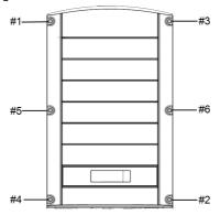
Figure 17: Tightening order of the screws
