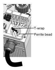
Figure 13: Attaching a Ferrite bead
