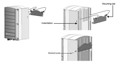
Figure 10: Hanging the inverter on the bracket
