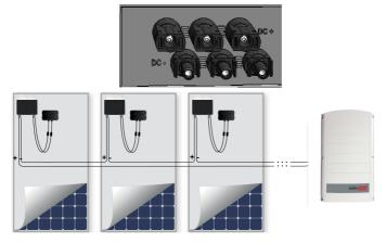
Figure 15: Inverter DC Connections
