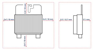
Figure 5: Power optimizer clearance
