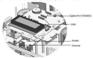
Figure 20: Internal connectors
