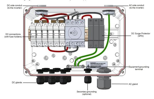
Figure 30: Inside the DC Safety Unit with fuses
