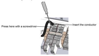
Figure 34: Spring-clamp terminals
