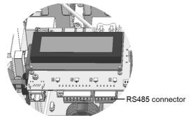
Figure 25: RS485 terminal block on the communication board
