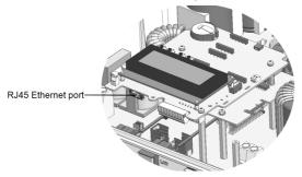
Figure 24: The RJ45 Ethernet connection
