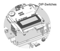
Figure 27: RS485 termination switch
