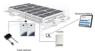
Figure 4: The SolarEdge power harvesting system components
