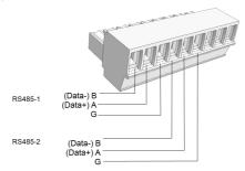
Figure 26: RS485 terminal block
