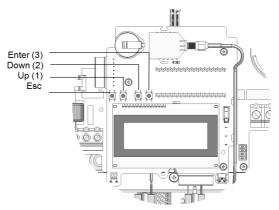
Figure 18: LCD Internal menu buttons
