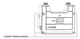
Figure 31: Opening the DC Safety Unit cover
