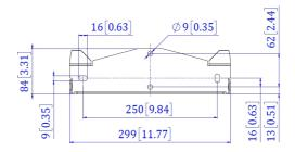
Figure 29: Inverter mounting bracket
